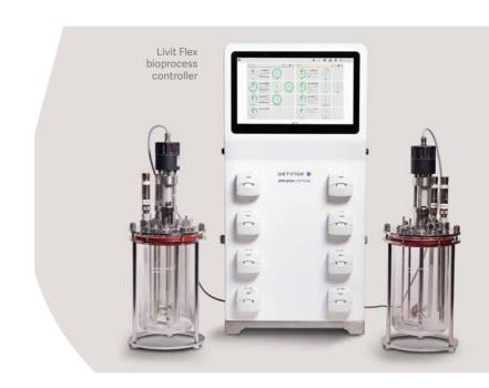
Livit Flex can be configured as a single or dual control system for single-use or multi-use bioreactors to optimize bench space in the laboratory. The new Livit Links enable plug-and-play connection of sensors and auxiliaries, with the controller automatically recognizing new devices.
