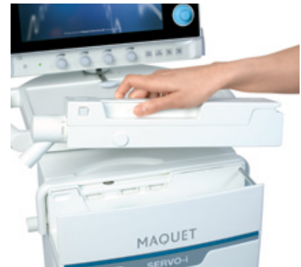
Servo-i interchangeable expiratory cassette
