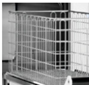
The perforated tray with rollers supports loading of modular wire baskets. For one wire basket (590 x 300 x 190 mm) or 2–3 baskets (590 x 300 x 100 mm), or a combination.
