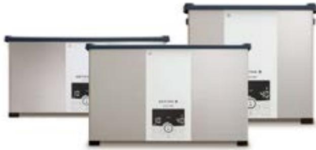
The range of Getinge Elmasonic Med Ultrasonic Cleaning units are freestanding bench models with stainless steel tank and are available in six different models, from 6 liters to 90 liters. Ultrasonic cleaning makes it possible to clean intricate parts with little or no disassembly, because ultrasound will clean wherever the cleaning liquid gets in contact with a surface. Including lid.
